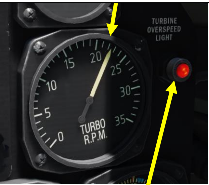
Turbine Overspeed Light
