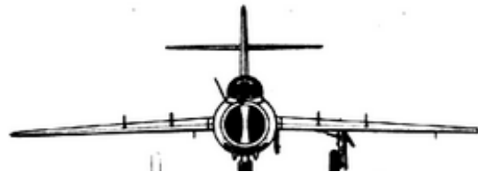
Wingspan of a MiG-15: 32 ft (10 m) (Value to enter in gunsight wingspan)
