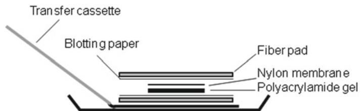
Fig. 3. Schematic representation of the transfer system described in this paper.
