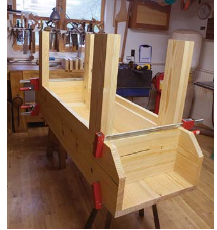
Can't miss II. With the top plate between the legs, you can put each stretcher on with screws (skip the glue because this is a cross-grain construction).
