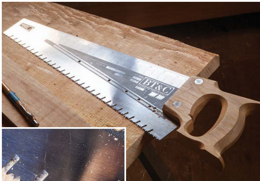
A great throwback. The Hardware Store Saw recalls some 20th-century saws that were packed with “features.” But these are useful (unlike a laser in the handle). A close-up shows the unusual tooth filing. Though it looks complex, it's actually not much more difficult to file than a standard crosscut saw.
