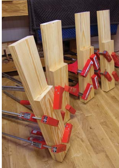
Four legs good. By gluing a short piece and a long piece together, you create a thick leg and the notch for the workbench's apron.
