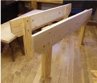
Legs & aprons. With the legs and aprons bolted together, you can glue up the parts for the benchtop.
