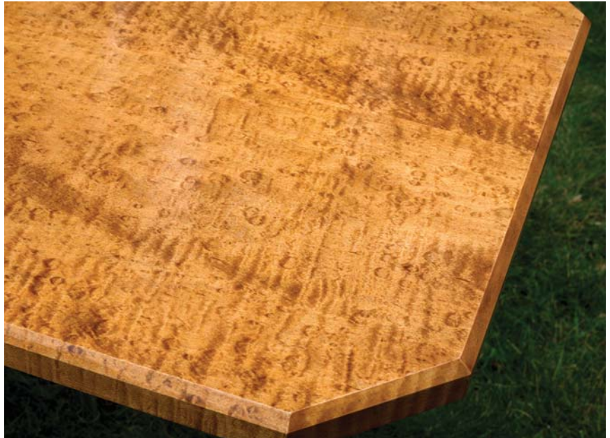
Small detail, big punch. A chamfer can transform an otherwise ordinary surface.
