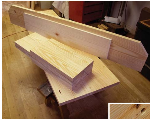
Aprons at work. Here you can see the 2x12 apron glued to the 1x10 interior piece. The legs will then butt against the 1x10.
