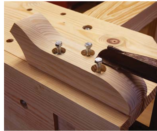
The hook. You can bolt your crochet on. Some early accounts indicate it was nailed on. You probably could get away with glue alone.
