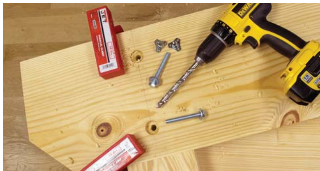
Mounting plates. Here is how the mounting plates look when they are installed. First you tighten the bolts, then you screw the mounting plate down. This way you can't miss.
