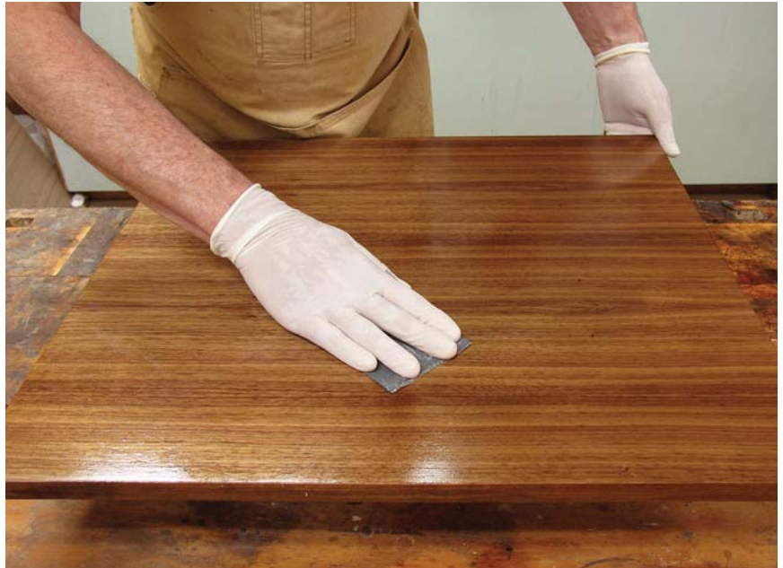
Smooth sailing. A project is not really finished until it's finished. A few simple shortcuts can help make finishing go smoothly, so to speak. For example, sanding oil finishes wet can save time.
