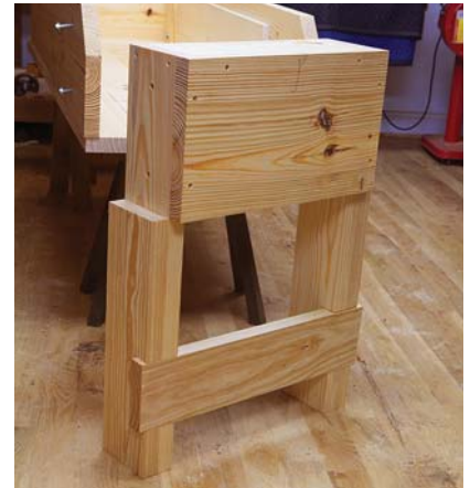
An end, assembled. I know this is an odd construction, but it works. And once you see it, you'll get it. Here you can see the finished end assembly with the lower stretcher ready for trimming and screwing.
