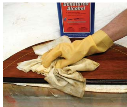
Soak it off. Remove shellac or lacquer with rags wetted with alcohol or lacquer thinner.
