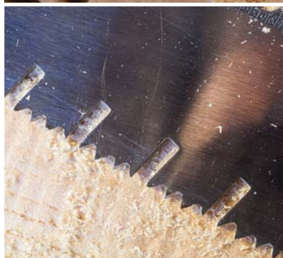
A great throwback. The Hardware Store Saw recalls some 20th-century saws that were packed with “features.” But these are useful (unlike a laser in the handle). A close-up shows the unusual tooth filing. Though it looks complex, it's actually not much more difficult to file than a standard crosscut saw.
