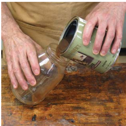
Made-to-order sheen. Create the sheen you want from a single can of satin finish.
