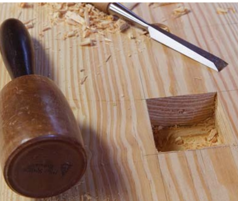
Square hole. This is a great first mortise for a beginning woodworker. Take your time in squaring up the walls.
