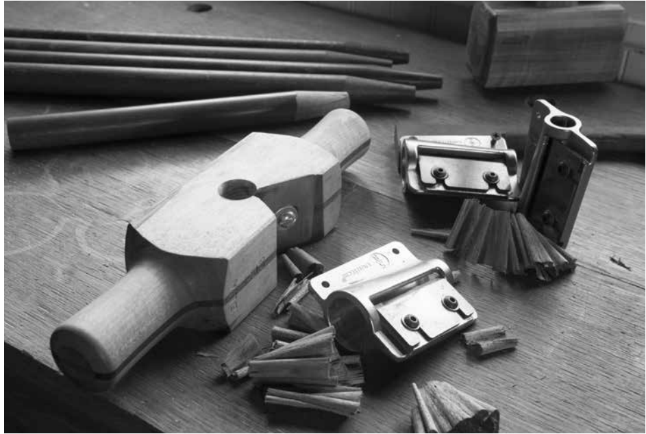
Two tenon cutters. While you can make your own tapered tenon cutter, it's faster to buy one. Here you can see a wooden version and metallic ones.
