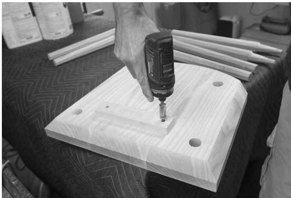
Easy seat. A temporary block on the underside – cheated toward the front edge of the seat – allows you to clamp the seat to plane it flat.
