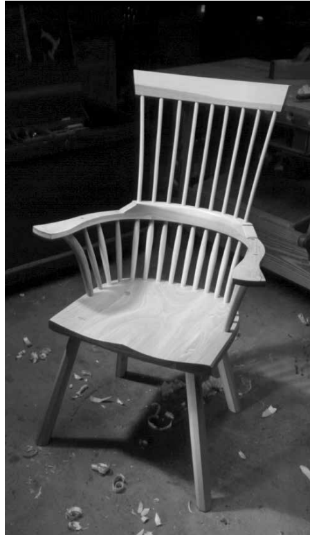
With & without. One of my Welsh stick chairs (left) built with staked joinery and stretchers in the undercarriage. A Welsh chair (right) without stretchers. And a three-legged backstool (below) without stretchers.
