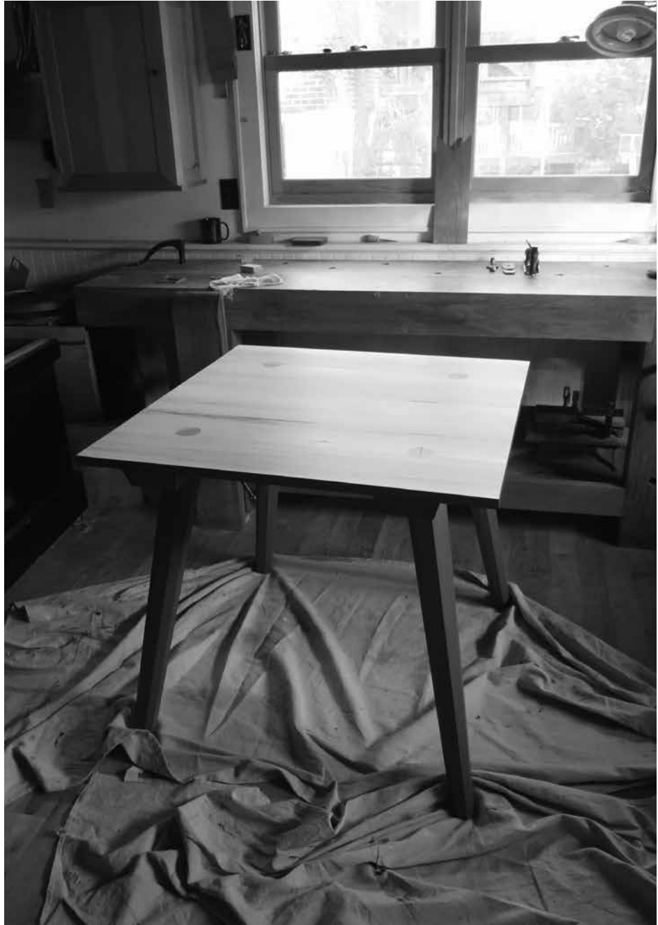
Really scrubbed. I used a soap finish on the top of this worktable. Four coats of soap resulted in a low-sheen finish.
