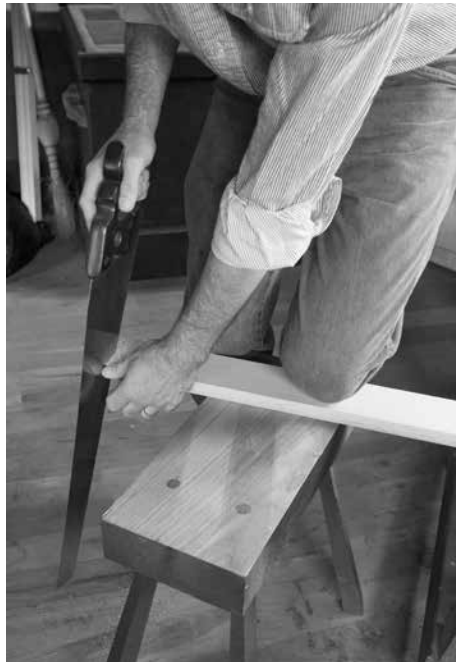
The first leg vise. One knee presses the work down. The other restrains the work from rotating.
