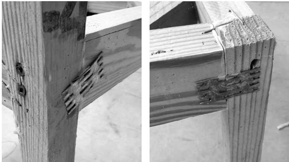
This is why we fight. Typical interior "joinery" on a modern upholstered chair.
