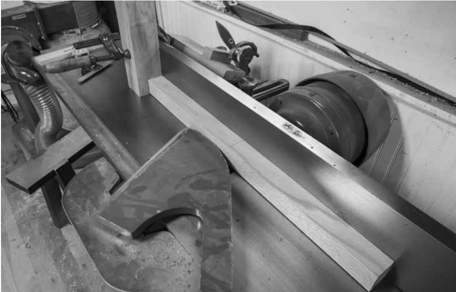
Set the stop. The leg should stop halfway along the taper.
