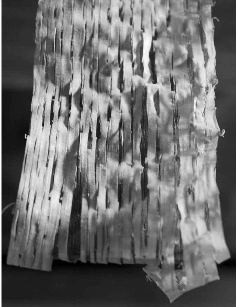
Poker straight. A shaving from a leg for a staked sawbench. The straighter the fibers, the stronger the component. This is true for chairs, ladders, tables and anything else that has to bear a heavy load.
