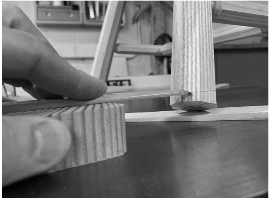
The half-pencil and a block of wood helps you mark out the correct length of the legs.
