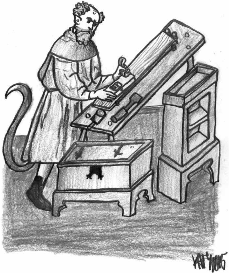
Roman workbench. Though this drawing is adapted from a 15th-century painting, the bench is Roman and uses staked joinery. The legs pierce the top without any stretchers or other reinforcement.
