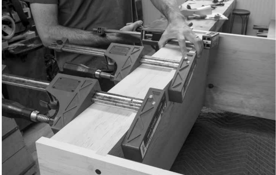
Long-grain kick. The kick is glued in place to the underside of the lower shelf. Then it is nailed in place through the sides of the bookcase.
