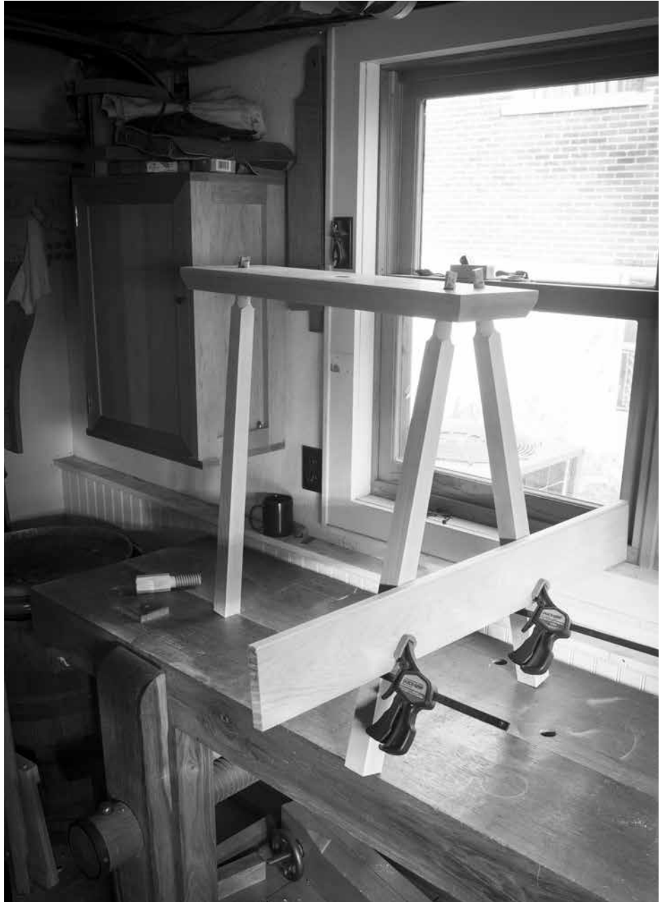
Clamped for success. The two clamps and flat board keep the front legs lined up during assembly.
