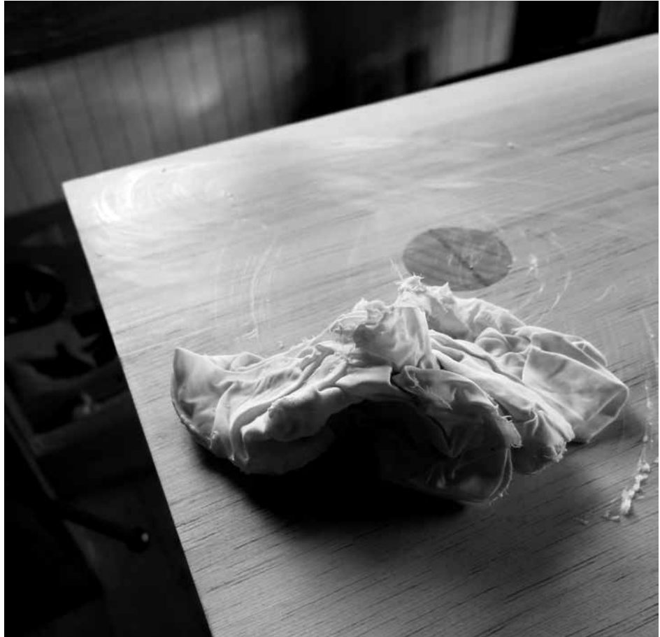
Soap's on. The thin soap finish rags on like a soft hand cream.
