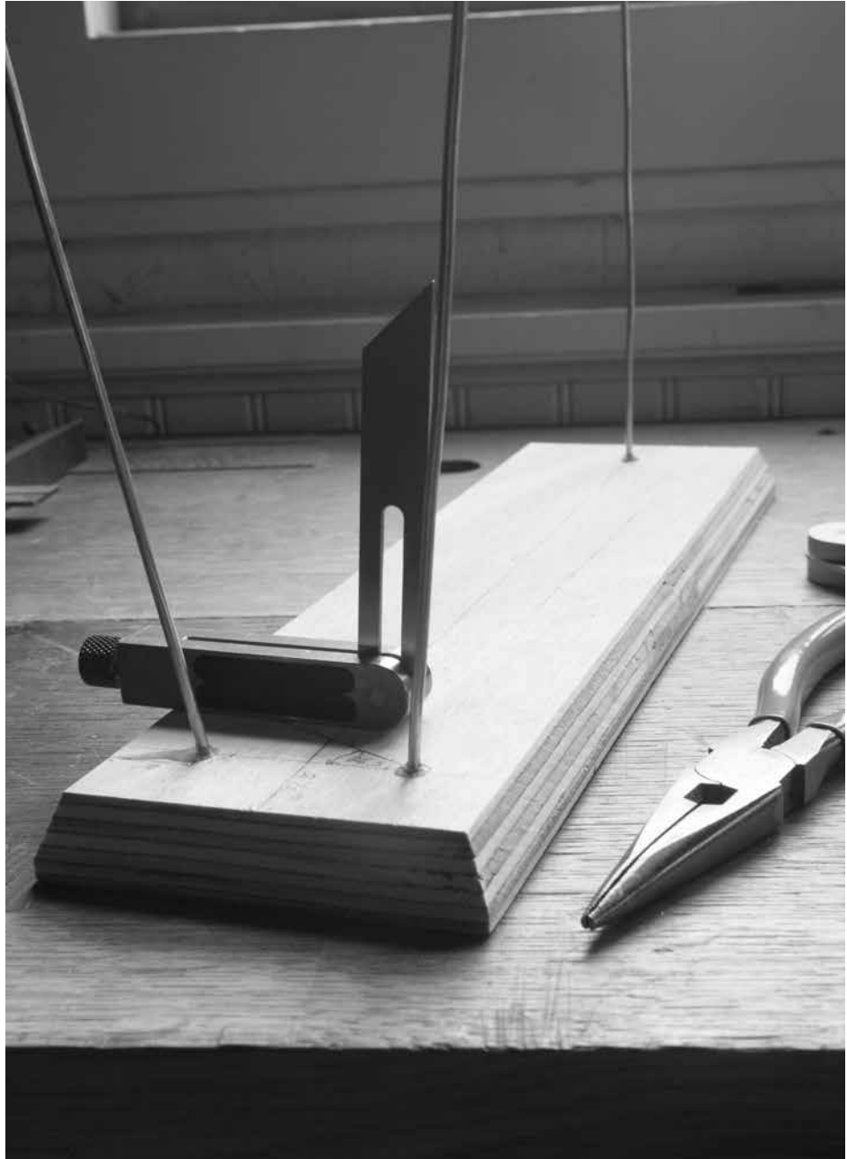
Real wireframe models. Alter the rake and splay with needle-nose pliers that are guided by a bevel gauge. Too much rake or splay here will create a tripping hazard.
