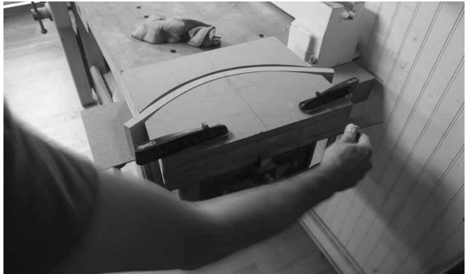
Screwed & bent. You can easily bend the crest in a form (the same form for the back-stool) by pressing the two halves of the form together on a workbench's vise.
