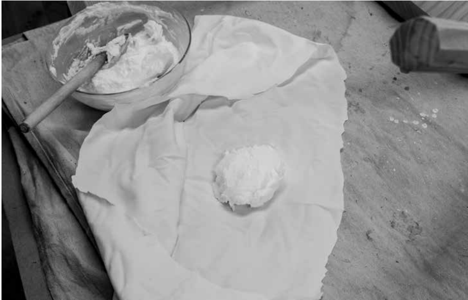
The whole ball of soap. Spoon the soap into a rag and wrap it around the ball to create something similar to a “rubber” when French polishing.
