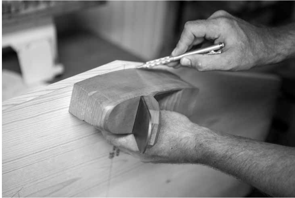
Two coffins. The boat shape of a coffin smoother is ideal for fairing the curves on the long edges of the bottom board.
