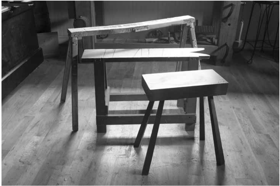
Saw-somethings. All these forms are made for sawing. The sawbenches are for hand-saws. The taller sawhorse is for electric saws.
