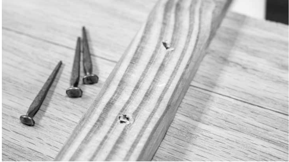
Not much to see. When done correctly, the tip of a clenched nail hits the metal surface and turns back into the work. What you see on the exit side is a rectangle of metal.
