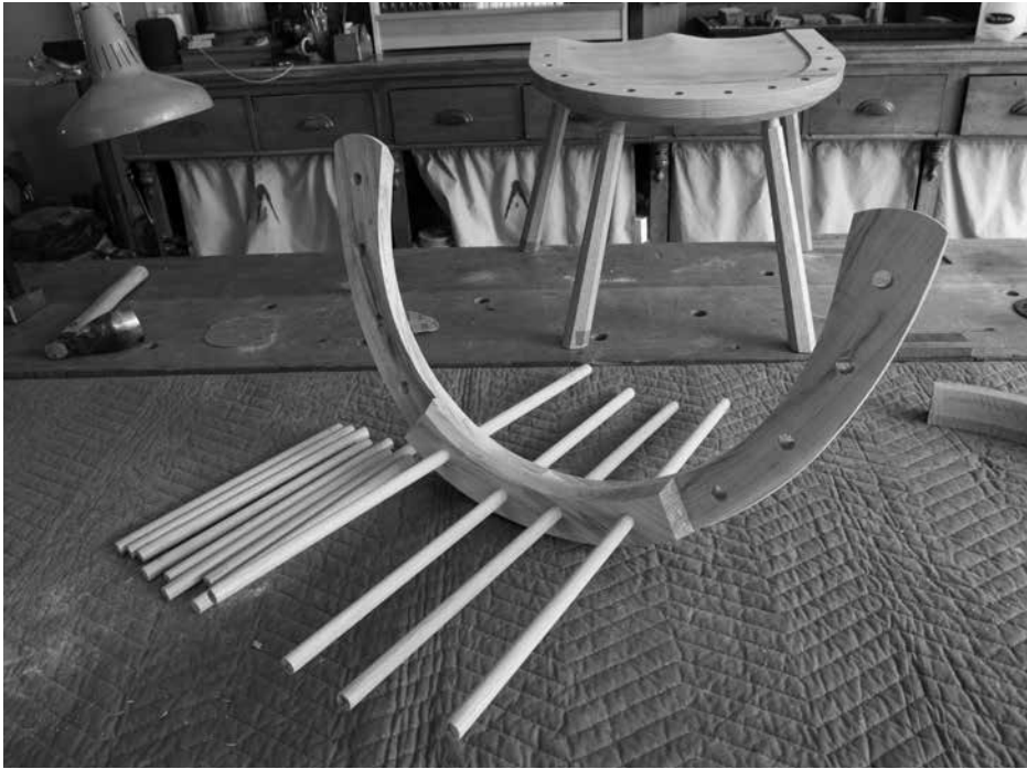
Fit sticks. Here you can see the back sticks that slide smoothly into the armbow.
