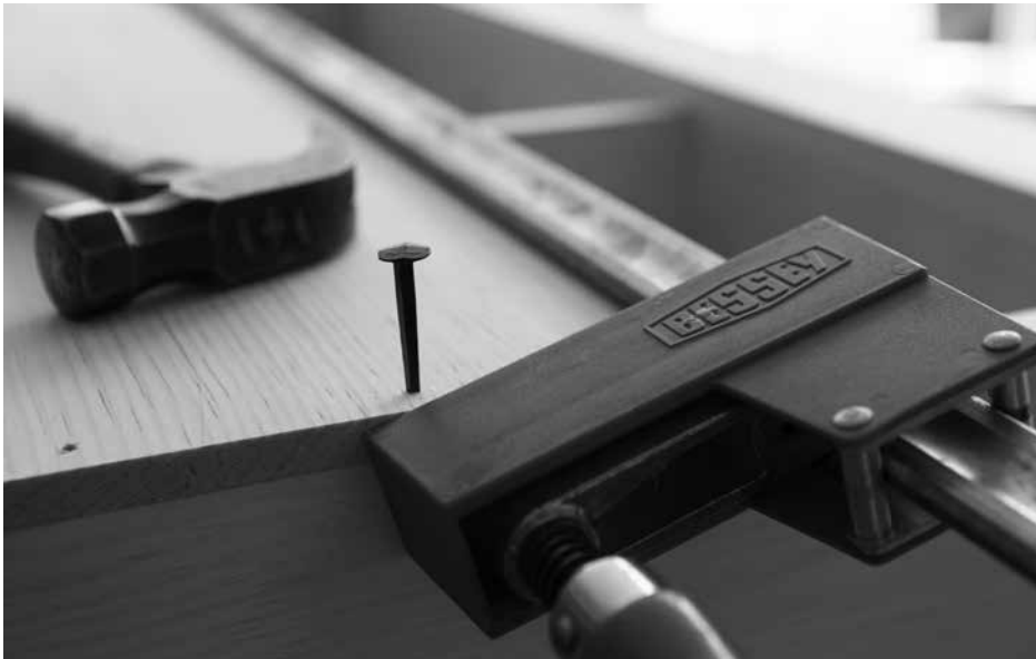
One clamp. Clamping the end grain – hard – helps prevent splits.
