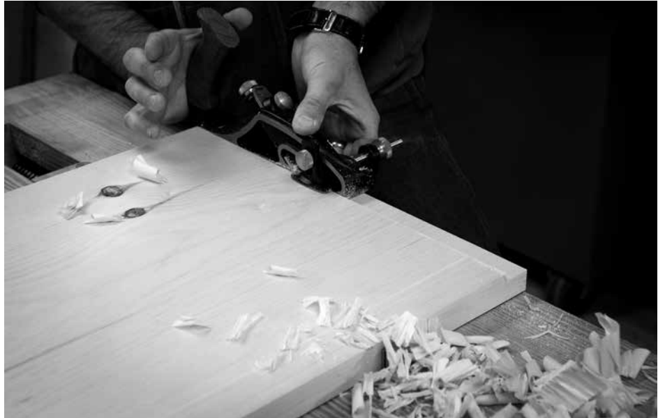
One of many ways. Cutting cross-grain rabbets can be done with a moving fillister (shown), a simple rabbet plane or even a shoulder plane.
