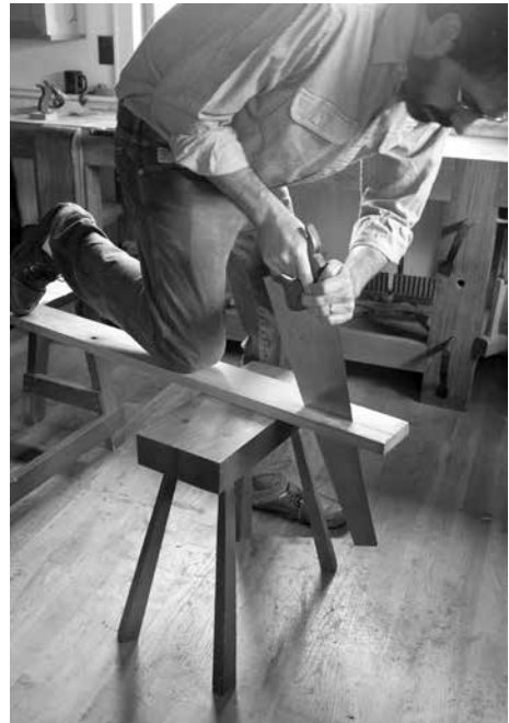
Ripping. This is an effective way to rip, but it does make my back sore.
