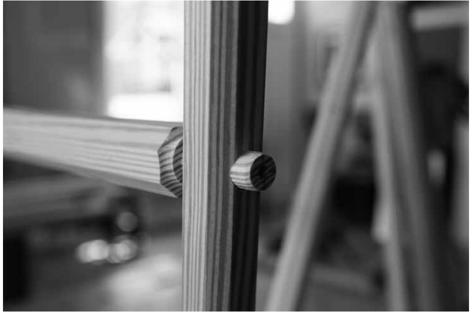
The joint. Here's the through-tenon after drilling. Not bad for freehand work.
